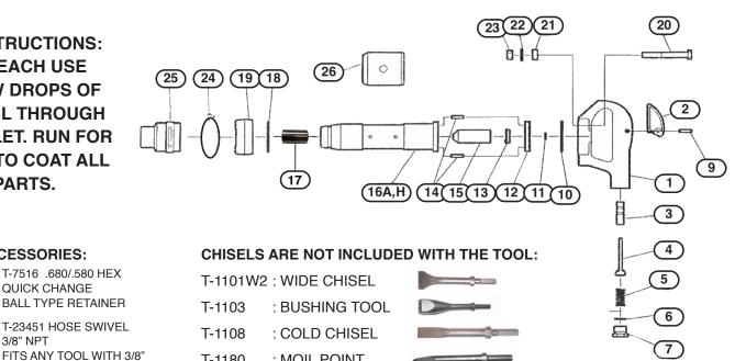
THESE CHISELS FIT OUR T-#24B, T-#34B, T-#44B, T-#2, T-#3 & T-#4 CHIPPING HAMMERS AS WELL AS ANY CHIPPING HAMMER THAT ACCEPTS .680 ROUND SHANK OVAL COLLAR CHISELS. FORGED STEEL. MADE IN USA. THE T-1103 IS 9 1/2" LONG. THE OTHER THREE CHISELS AVAILABLE IN 9", 12", OR 18" LENGTH. .580 HEX CHISELS ALSO AVAILABLE FOR "BH" HAMMERS
